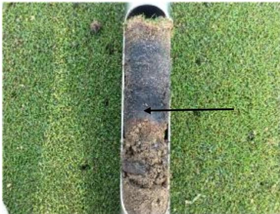
Figure 9: Inspection of the soil profiles beneath the greens highlighted the same issues across the course. We could see a silty material at depth which has been imported during the original turfing of the greens (see arrow). This is restricting the movement of water to the underlying sandy construction material. Note the blackening of the soil in the photo highlights where water is being retained in excess.
