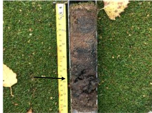
Figure 10: The depth of this silty layer did appear to vary across the course, with it being nearer to the surface on newer greens (e.g. back 9) but deeper on older greens where a greater build-up of topdressing can be seen. See picture above from beneath the 8<sup>th</sup> green where the layer is occurring at 6 – 7 inch depth.
