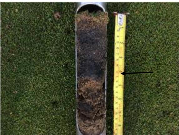
Figure 11: On greens such as the 16<sup>th</sup> we can see that the silt layer is much shallower at 4 inches. This will have a negative impact on drainage but will be easier to remedy.
