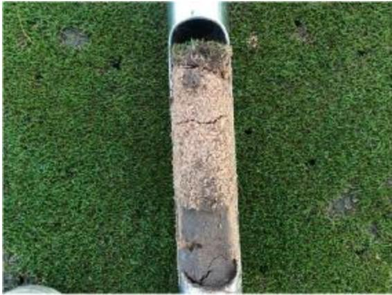
Figure 19: Further drainage installation is planned for next year on the notoriously poorer draining 8<sup>th</sup> and 16<sup>th</sup> greens. This is fully supported, however we discussed some slight alteration to the techniques and materials used. This was mostly lifting the turf prior to trenching (to minimise surface damage) and the use of a sand/soil mix instead of straight sand (to avoid turf droughting over drain lines in summer).
