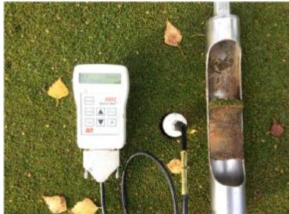
Figure 14: We carried out a simple test using a soil moisture probe on the 8<sup>th</sup> green to illustrate the impact of organic matter and found a 35% reduction in moisture content when the thatch layer was removed.
